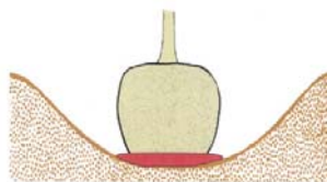
Figure 17. Stabilize the tree by firming a small ring of backfill soil around the base of the root ball.
